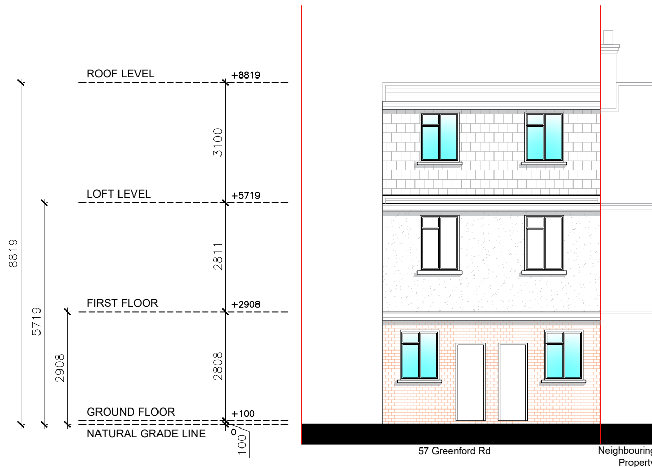
SOUTH-EAST ELEVATION (REAR VIEW)
